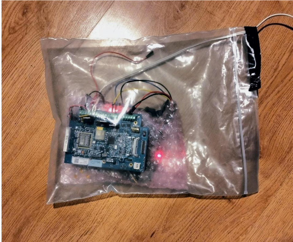
Figure 3 Photo of HW setup 1 (Bare PCBA) without enclosure
